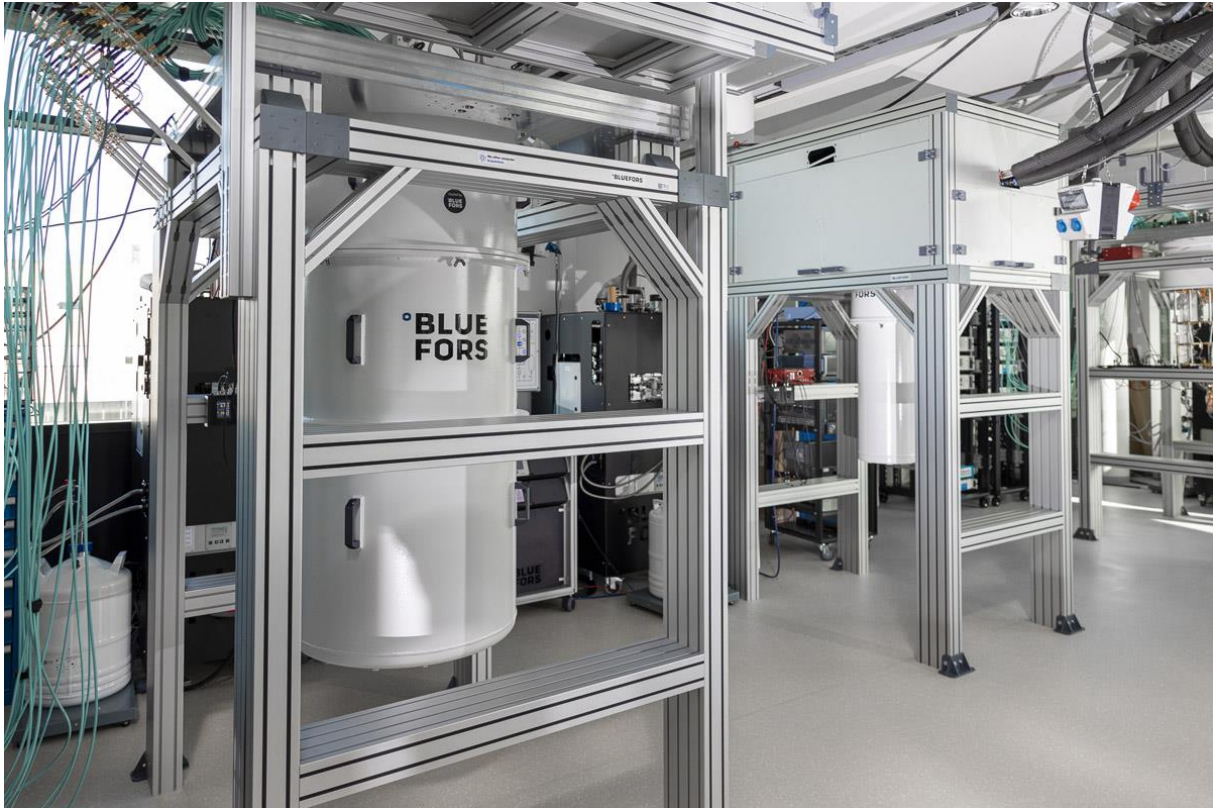
Cryostat in which the central unit of the QSolid prototype is cooled
